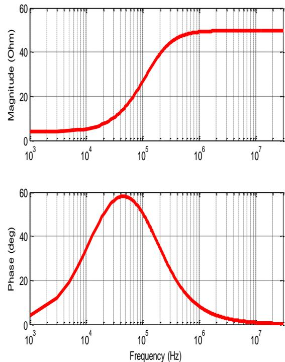
Fig. 5. LISN common-mode impedance
