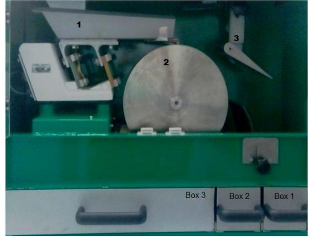
Fig. 3. Photography of roll type electrostatic separator.
