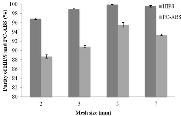
Fig. 4. Purity of HIPS and PC-ABS products
