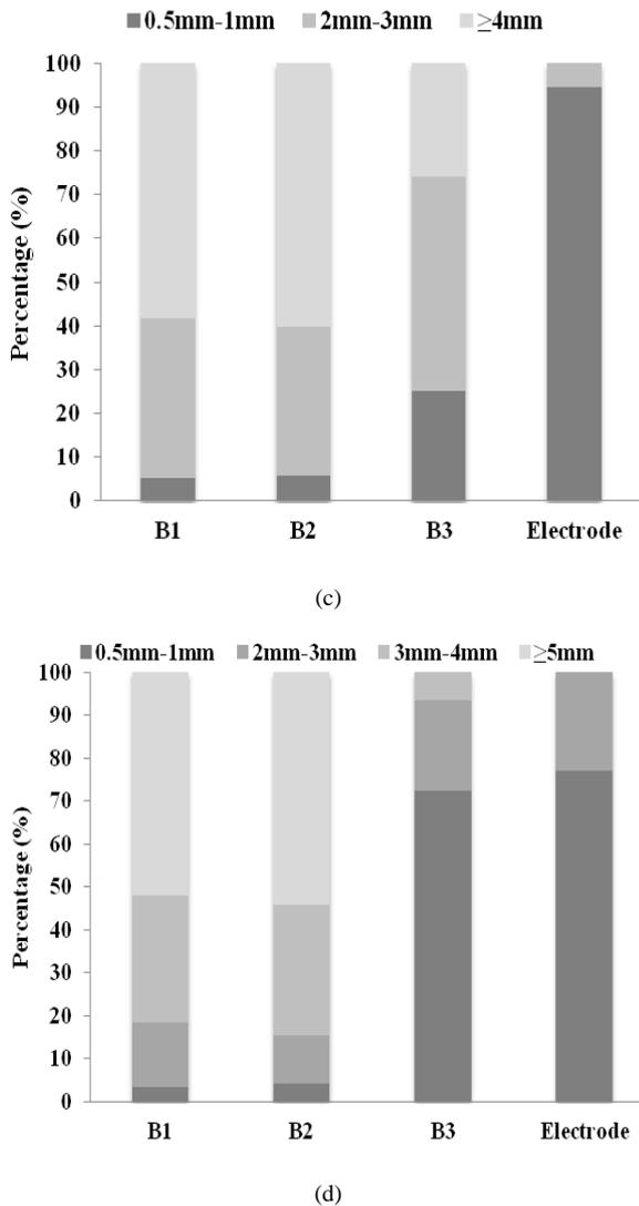
Fig. 6. Size distribution of particles in the collecting boxes (B1, B2, B3) and the electrode for different screen mesh diameters : (a) 2mm, (b) 3mm, (c) 5mm, (d) 7mm.
