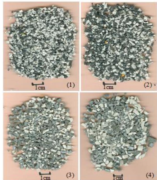
Fig. 2. Particle of PC-ABS and HIPS obtained after grinding : (1) using 2mm grid size; (2) 3mm grid size; (3) 5mm grid size; (4) 7mm grid size.
