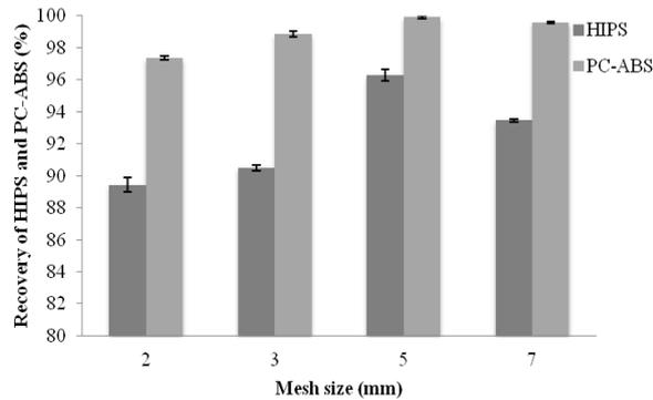
Fig. 5. Recovery of HIPS and PC-ABS products
