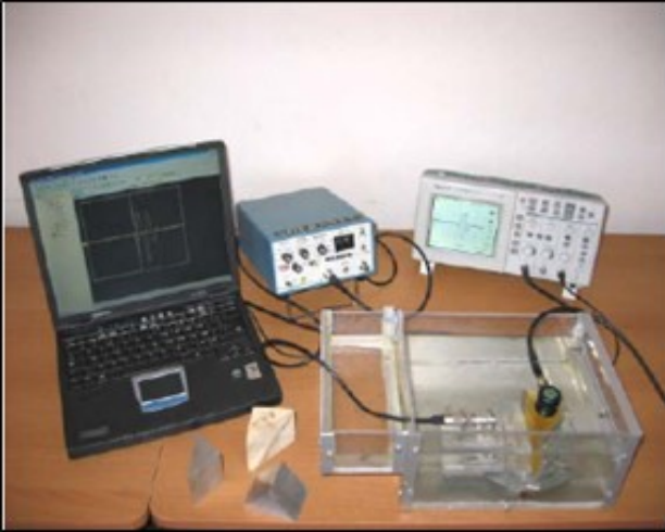
Fig. 2. Measurement device of immersion technique.
