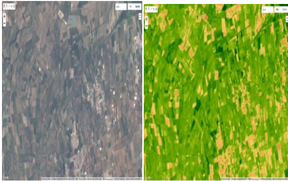
Fig. 2. Image showing RGB and NDVI for the coordinate center (2.78498, 36.57439) using Google Earth Engine.
